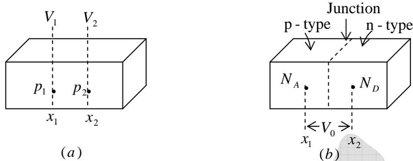
**Figure (a):** A graded semiconductor:  $p(x)$  is not constant
